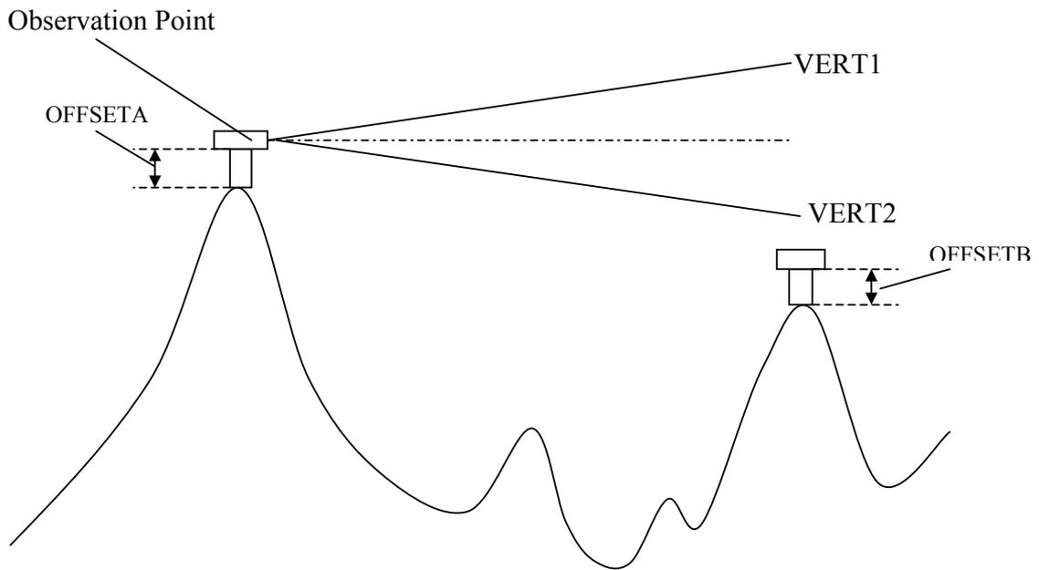
**Figure 4: Parameters required by the Visibility request in the software ArcView (Top View)**
