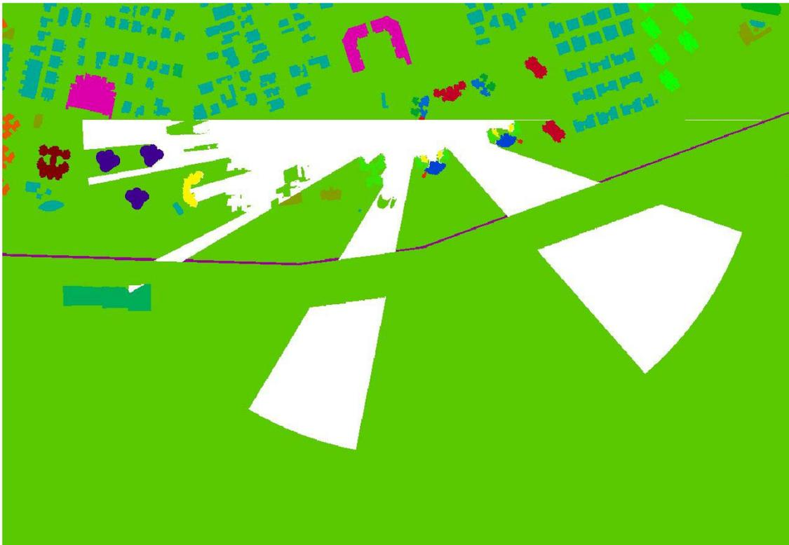
Note: The portion in white represents the viewshed. The different color schemes in the grid output represent the different elevation height of the study area.
