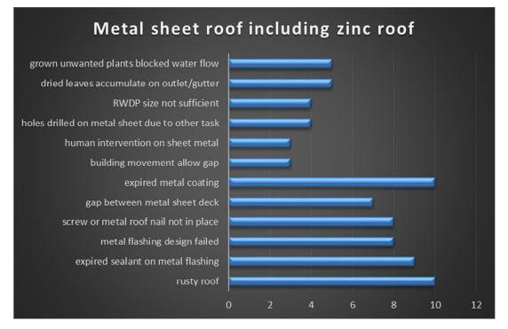
The next one is the problem arises when the sealant become not function or expired especially along the metal flashing and become permits water. Improper installation of metal flashing to the existing metal roofing always permit water seep through the leakage points and giving problem to the structure.
